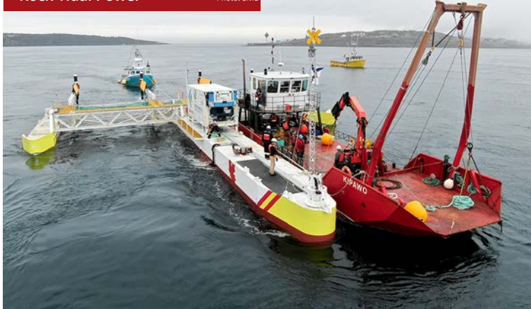
JOINT VENTURE: Sustainable Marine Energy's Plat-I device installed in the Grand Passage of Nova Scotia in Canada for Black Rock Tidal Power
