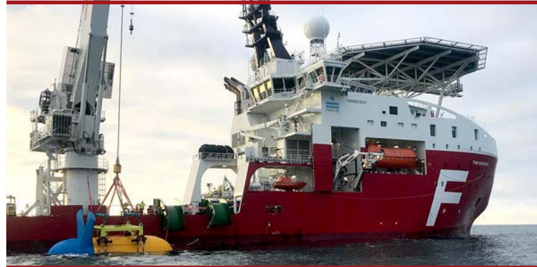
PASSAGE OF TIME: Sabella redeployed its upgraded D10 1MW tidal turbine off Brittany in October Photo: Sabella
